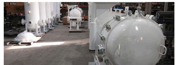
Filtration vessels in fabrication: sampling connections, differential pressure indication, air release and full drain provisions.
